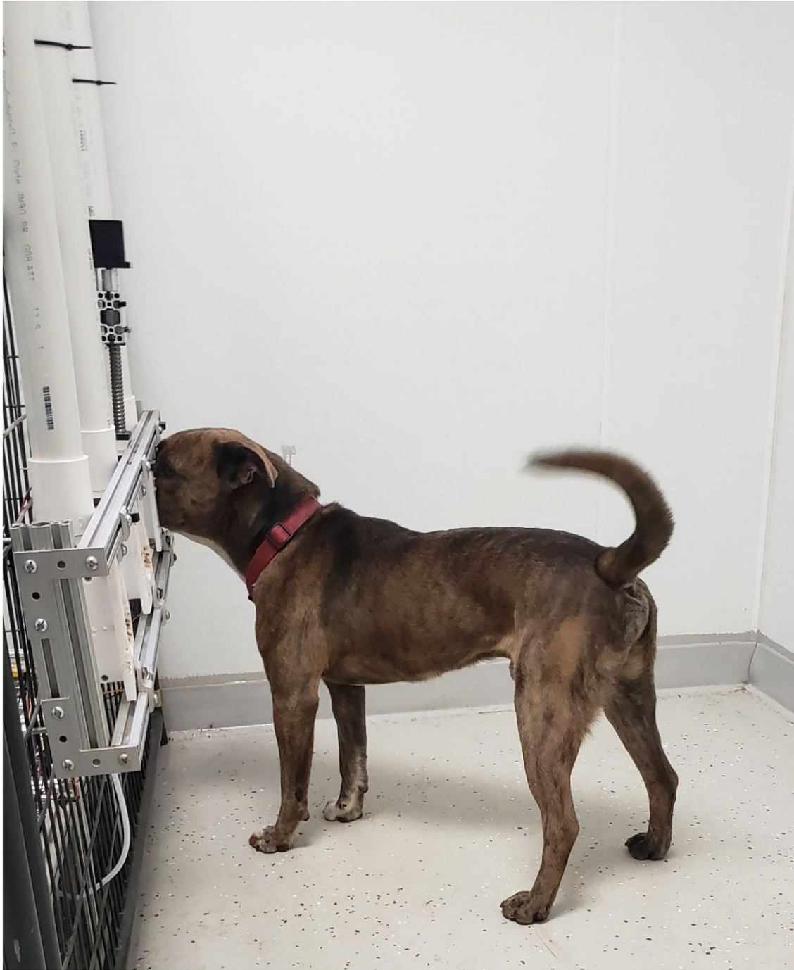
FIGURE 3 | Buster Alerting to the port containing the target odor. Infrared (IR) sensors located at the front of the port measure the nose hold duration, providing an objective recording of the dogs' alert.
