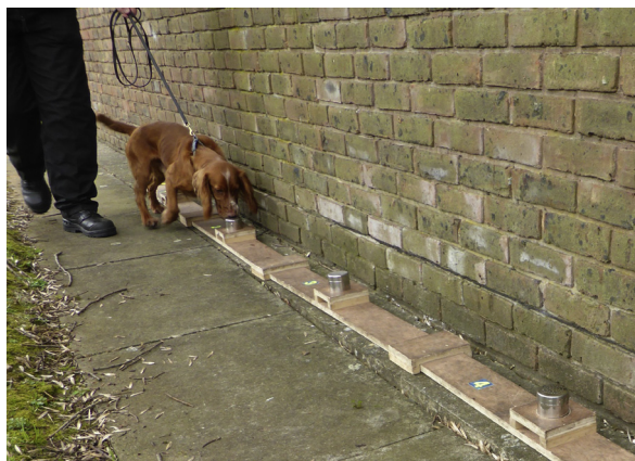
Fig. 1. Odour ID test set up showing first four stands and removable stainless steel tins.
